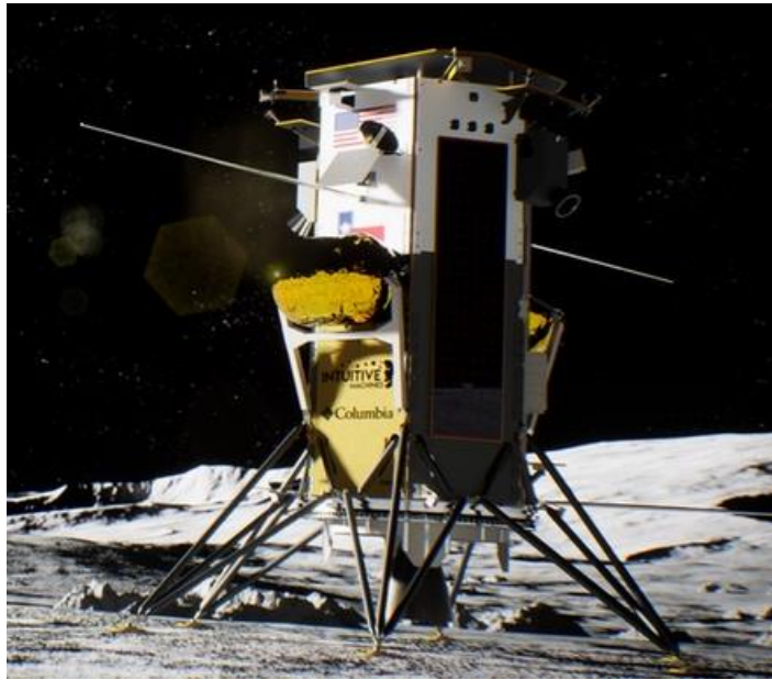
IM-1 with ROLSES antennas deployed
