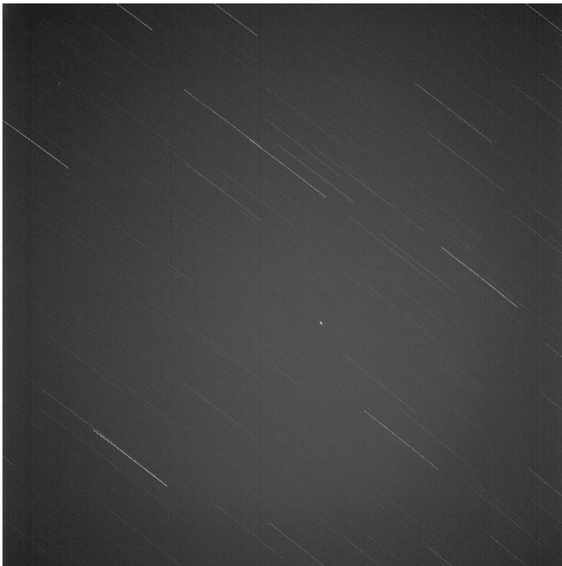
Figure D.2.6. Starlink-1130 being tracked by the POMENIS Observatory on 16 May 2020. The background stars are severely streaked and often overlap making photometry and astrometry difficult to do accurately.
